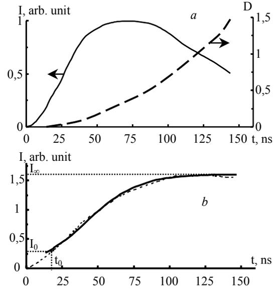
Fig. 5. Kinetics of  $\text{AgN}_3$  whisker explosive luminescence ( $\lambda = 550 \text{ nm}$ , the initiation was performed by laser pulse)
