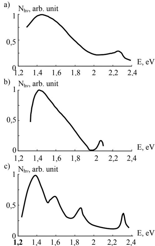
Fig. 4. HMA predetonation luminescence spectra of  $\text{AgN}_3$  (a),  $\text{Pb(N}_3)_2$  (b),  $\text{TiN}_3$  (c)
