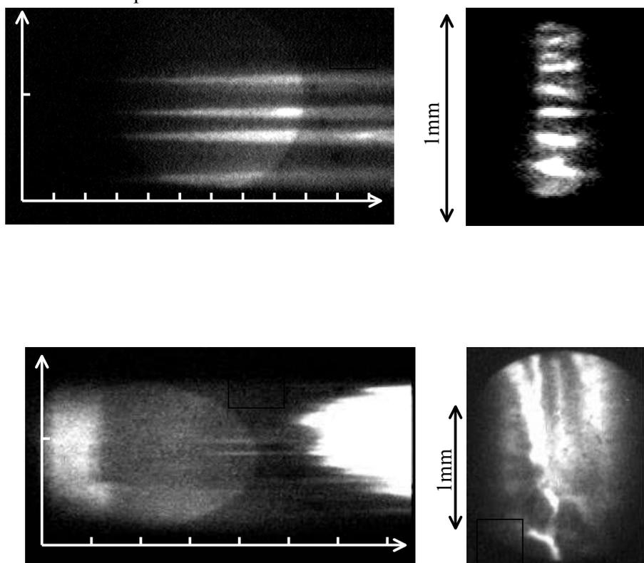
An enlarged image of silver azide whisker was transmitted by optical objective to photoelectric cathode of streak-camera "View 2A". Spatial resolution was 50  $\mu$ m.
