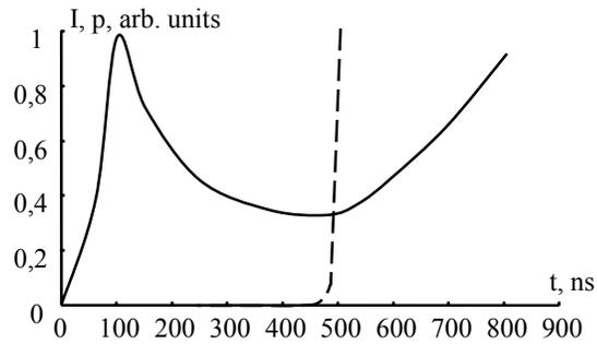
Fig. 3. Kinetics of  $\text{AgN}_3$  whisker explosive luminescence ( $\lambda = 550 \text{ nm}$ , the initiation was performed by laser pulse, crystal was mounted on a flat cell in contact with acoustic detector), solid line – light signal, dotted line - leading edge of acoustic signal..
