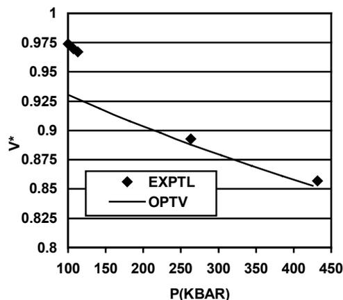
FIGURE 8.  $V^*$  VS  $P$  FOR Al OXIDE ( $\rho=3.812$  g/cc)
