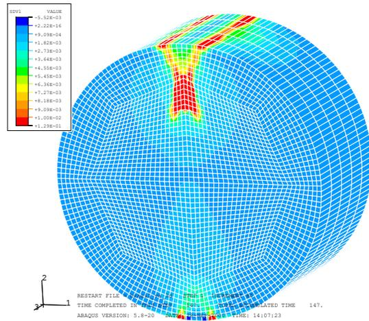
**Figure 4** The strain distribution calculated with ViscoSCRAM does not match experiments though.
