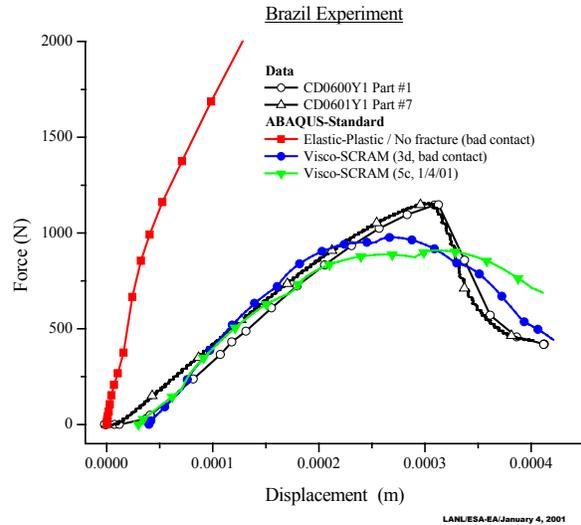
**Figure 3** Load deflection for Brazil test is a difficult test. Note that elastic plastic model simply dies, while ViscoSCRAM follows post peak unloading.
