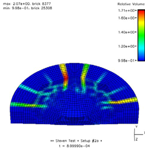
**Figure 5 Shows strain localization from fracture behavior in the elastic-plastic explosive model.**
