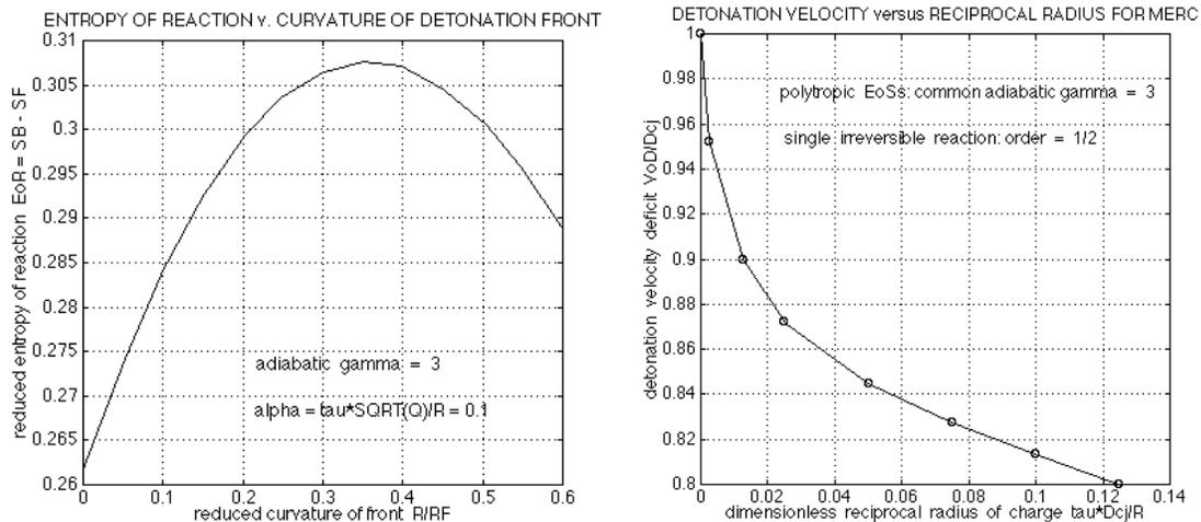
FIGURES 1 & 2. PLOTS FOR A POLYTROPIC EXPLOSIVE WITH ORDER OF REACTION  $M=1/2$  AND PRESSURE INDEX  $N=0$ , OF (1) THE GLOBAL ENTROPY OF EFFECTIVE REACTION (GEOER) AS A FUNCTION OF THE OF THE SHOCK FRONT CURVATURE FOR FIXED RADIUS  $R$  AND FIXED VOD, SHOWING A MAXIMUM; (2) THE VOD AS A FUNCTION OF RECIPROCAL RADIUS FOR GEOER OPTIMIZED WITH RESPECT TO THE CURVATURE OF THE SHOCK FRONT (IE. "SIZE EFFECT" PLOT)
