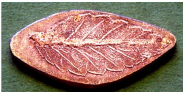
FIGURE 8. LEAF ENGRAVED IN COPPER BY THE MUNROE EFFECT.
