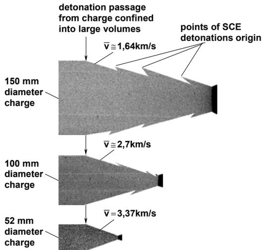
**FIGURE 5. SCHEMATIC VIEW OF EXPERIMENTAL STREAK-CAMERA RECORDINGS OF THE SOLUTION'S DETONATION PROPAGATION WITHIN LARGER VOLUMES OF THE SOLUTION AFTER ITS PASSAGE FROM CHARGES CINFINED INTO THE VOLUMES.**
