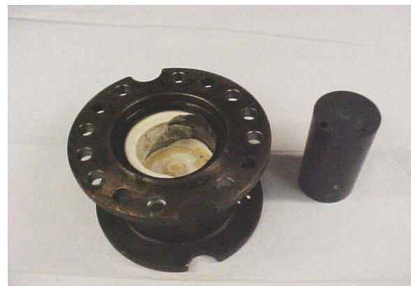
Figure 3. Melt cast system showing the plugging and the breakaway
