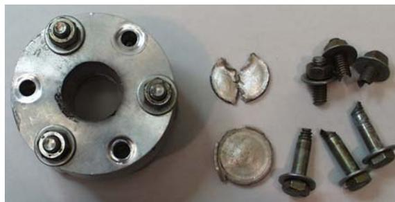
**FIGURE 8. RESULTS OF A COOK-OFF EXPERIMENT WITH PBX-9501 AT 198°C AND 9.6% EXPANSION VOLUME.**
