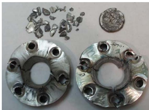
**FIGURE 9. RESULTS OF A COOK-OFF EXPERIMENT WITH PBX-9501 AT 192°C AND 9.6% EXPANSION VOLUME.**
