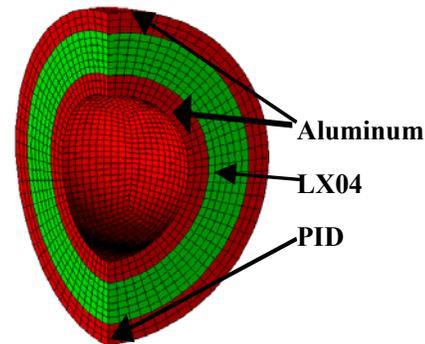
**Figure 3. Initial configuration of the spherical shells deflagration example.**
