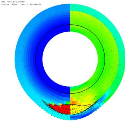
**Figure 4.** A slice through the spherical shells deflagration example shortly after initiation of deflagration. The log of the temperature between 350 K and 2000K is displayed on the left and the pressure between +/- .3 Gpa is displayed on the right. The internal circle is boundary between the inner aluminum shell and the unreacted explosive. The other line is the boundary between the reactant and product phases. The relative velocity field is also displayed.
