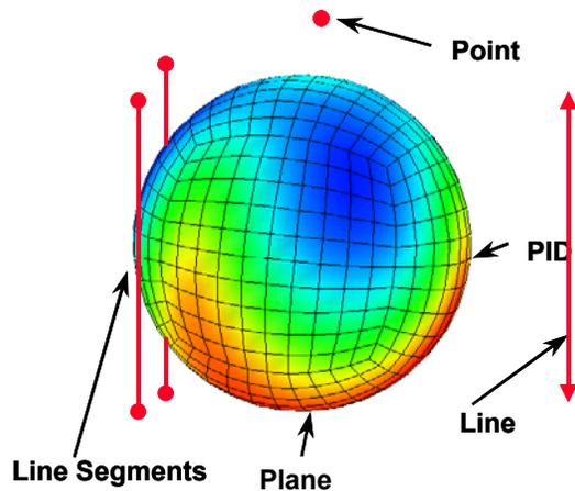
Figure 1. Example of a thermal profile on an aluminum sphere provided by a point source, line source, two line segment sources and a plane source, all controlled by a PID controller.
