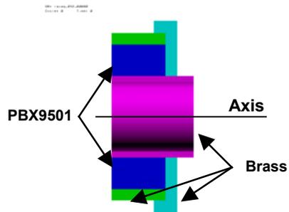
**Figure 5.** The initial material configuration of the Los Alamos Annular Cookoff Test. The pink, green and light blue regions are the brass, and the dark blue region is the unreacted explosive. The system is symmetric about the left side.
