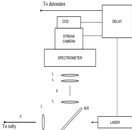
**FIGURE 2. SCHEMATIC DIAGRAM OF THE OPTICAL COMPONENTS USED TO COLLECT TIME RESOLVED FLUORESCENCE SPECTRA FROM THE FIBER SENSOR. CCD – CHARGE COUPLED DEVICE DETECTOR, F – OPTICAL FIBER, L – LENS, B/S – BEAM SPLITTER**
