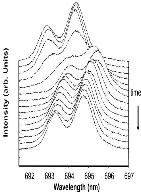
**FIGURE 3. TIME-RESOLVED SPECTRA WITH 70 NS RESOLUTION SHOWING MARKED IMPROVEMENT IN SIGNAL COLLECTION. EVEN WITH THE IMPROVED TIME-RESOLUTION, THE SIGNAL TO NOISE QUALITY IS BETTER THAN THAT COLLECTED FROM PREVIOUS SYSTEMS.**
