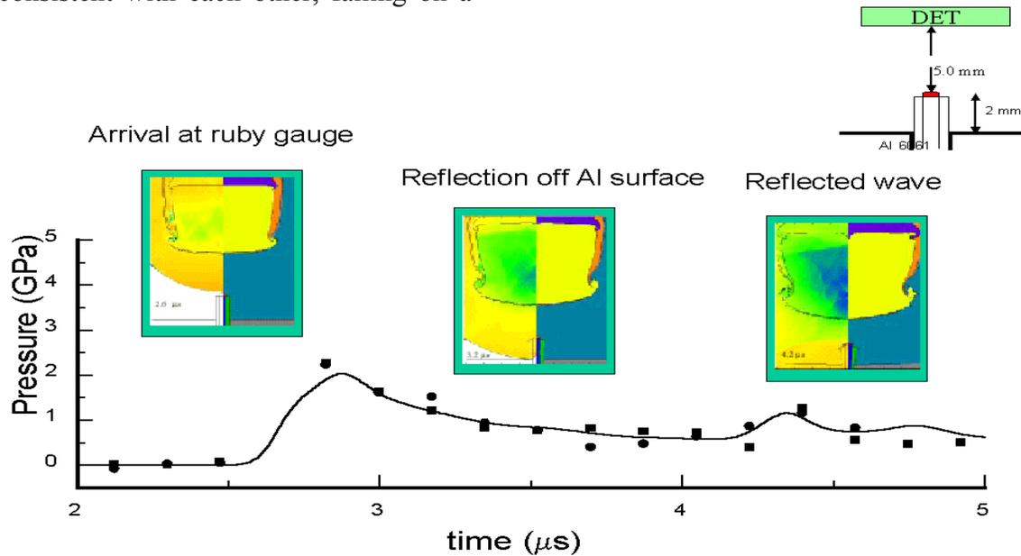
**FIGURE 5. PRESSURES DEDUCED FROM SPECTRA TYPIFIED BY FIGURE 4, AND THE AGREEMENT WITH CTH PREDICTIONS. POINTS ARE OBTAINED FROM DATA, WHILE THE CURVES ARE FROM CTH PREDICTIONS. UPPER INSERT SHOWS SPECIFIC GEOMETRY WHERE SENSOR PROBES THE SHOCK FROM THE DETONATOR, AND ITS REFLECTION OFF THE AL TARGET, WHILE PICTURE INSERTS SHOW CTH SNAPSHOTS OF THE SHOCK EVENT AT THE CORRESPONDING TIMES INDICATED BY ARROWS.**
