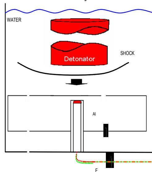
**FIGURE 1. SCHEMATIC DIAGRAM OF THE AQUARIUM CONTAINING THE DETONATOR AND THE RUBY SENSOR AT THE TIP OF THE FIBER IMBEDDED IN THE AL TARGET.**
