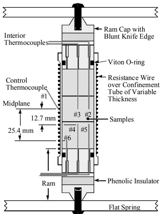
**FIGURE 2. DETAILS OF TEST CELL**
