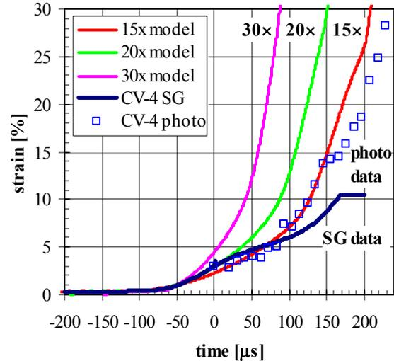
**FIGURE 7. COMPARISON OF MODEL AND EXPERIMENT IN PBXN-109 SHOT CV-4**
