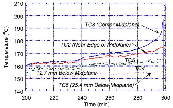
**FIGURE 3. TEMPERATURES IN PBXN-109, SHOT CV-2**
