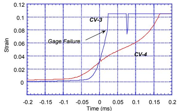
**FIGURE 4. TUBE STRAIN DURING COOK-OFF IN SHOTS CV-3,4**
