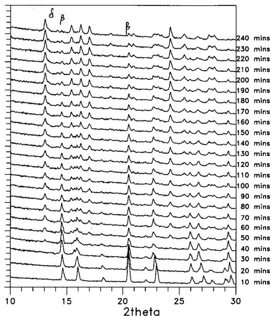
Figure 4: XRD patterns of kinetic study of coarse HMX
