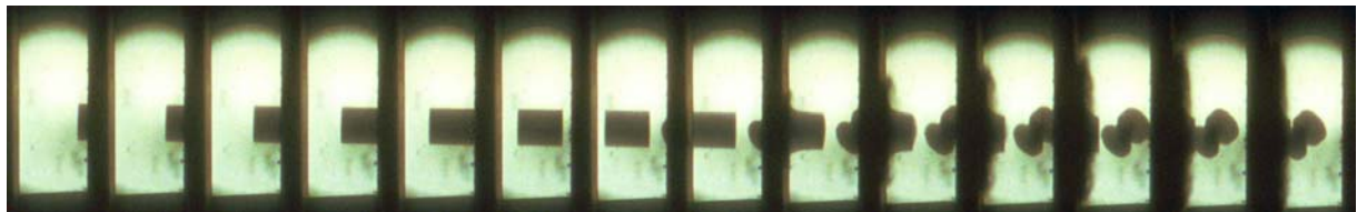
Figure 5: Impact of 9 gram, 18 mm diameter HU-43 cylinder on steel, at an impact velocity of 145 \text{ ms}^{-1} .
