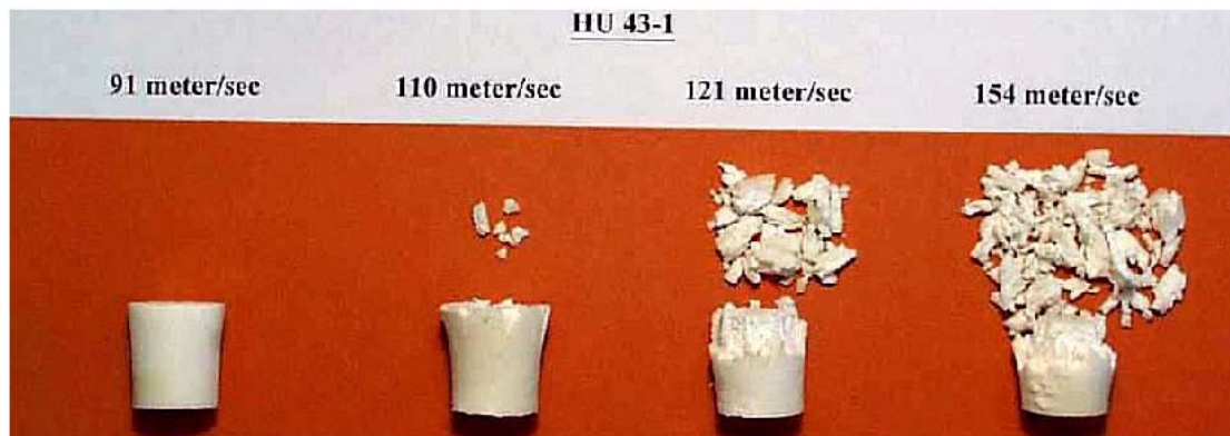
Figure 4: Fragments of HU-43 collected after firing bare cylinders on a steel plate at indicated velocities.
