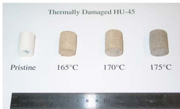
Figure 12 a: Thermally damaged samples of temperatures of respectively 165, 170 and 175°C (for 5 hours) compared to pristine material
