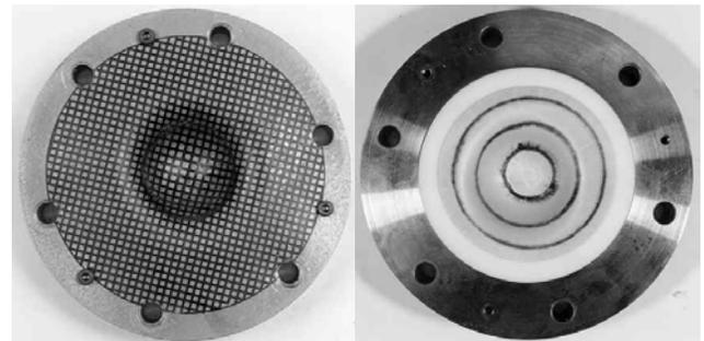
**Figure 3** Low speed impact on configuration 1
