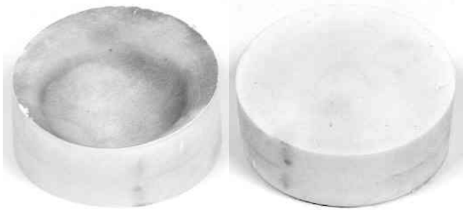
Figure 6 An explosive puck retrieved from double thickness impacts.
